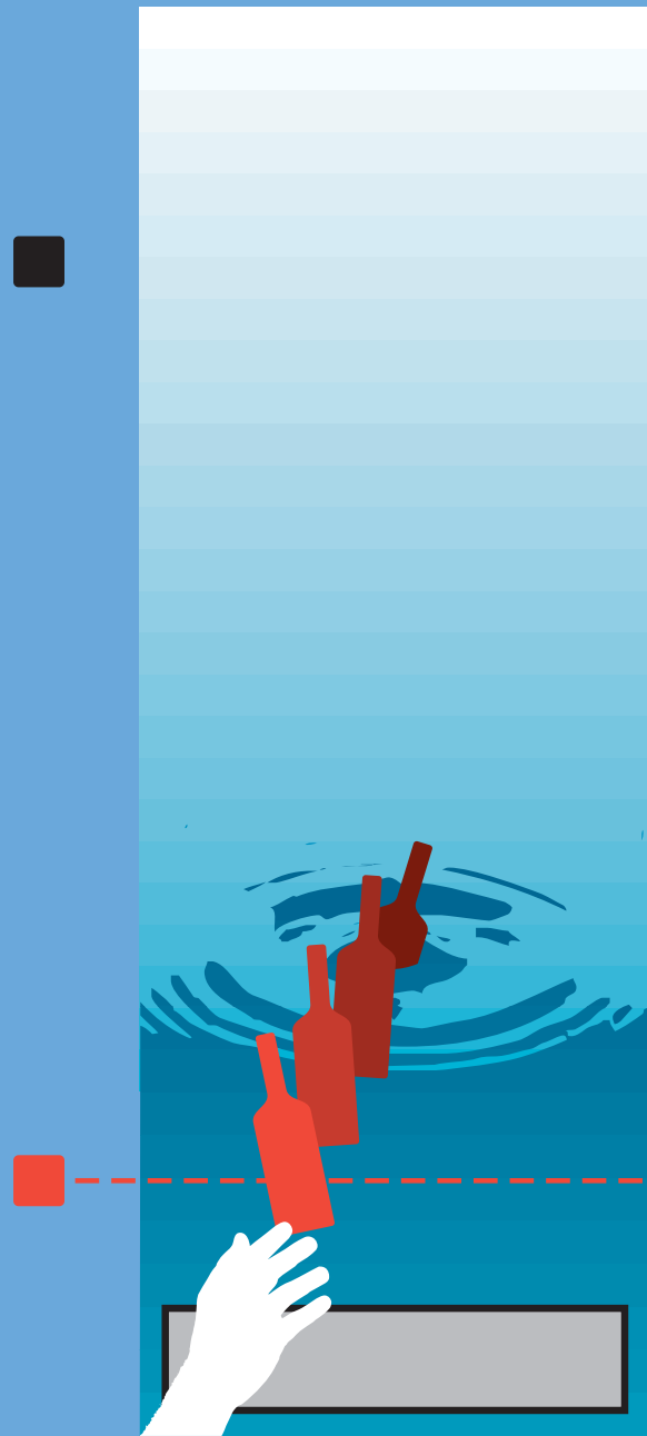
The user throws the floater beyond the first line of sensors: the magnets start moving
