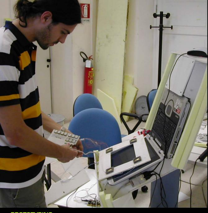
The **prototyping** proceeded with the realization of the **structure** of the device, the four **buttons**, the **screen** and the **identification system**. A multimedia animation software was used to create a simple interface.
